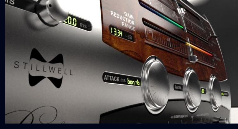
Manual/Variable Release Time: A constant release time can be dialed in with the control, which is continuously variable from 1 to 2000 milliseconds. Ideal for fine control over material with closely predictable dynamics, such as single tracks, electronica and rock mixes.
